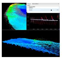
The Sonar Noise Classifier is trained to identify a variety of noise patterns from acoustic sensors. The algorithm assigns confidence values for all soundings on a scale of 0 to 100% with 100% indicating the classifier's highest confidence that the sounding is noise. Soundings can
