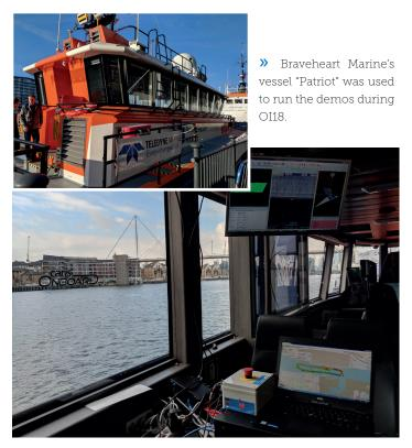
» Image aboard the Patriot, showing Teledyne PDS controlling the sonar in the top screen, and CARIS Onboard displaying the automatically processed surface on the bottom screen. This demonstrates how the processed data can be used on the vessel to guide the hydrographer without distracting from running the survey equipment.
