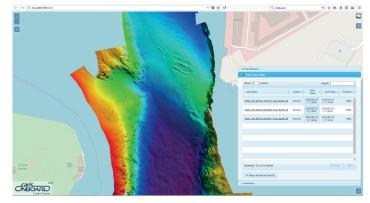
» CARIS Onboard 2.0 Control Centre is opened in a web browser. It is focused on a web-map which provides real-time survey visualization, in addition to the tools for controlling data processing.
